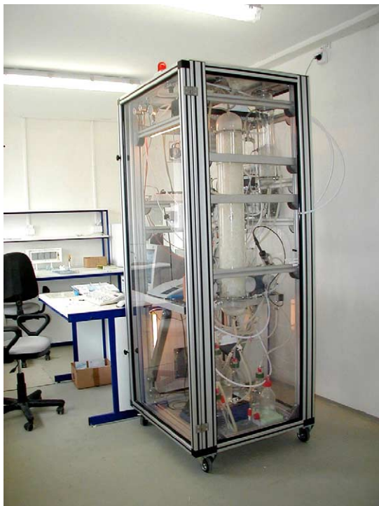
Fig. 4. Biological H 2 S removal unit developed by Profactor, in the fuel cell lab from Uni Nitra (Slovakia).
