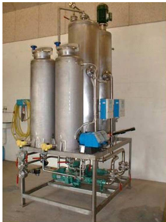
Fig. 5. Chemical H 2 S removal unit developed by Seaborne.
